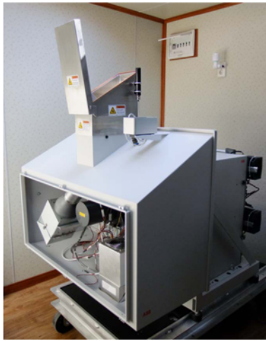
Fig. 4. AERI system located inside secure container. The light path from the door on the roof to the selection mirror of the AERI system is about 140 cm.
